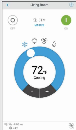
**Control and monitor indoor unit's ON/OFF, mode, set-point, fan speed, room temperature, and error status.**
